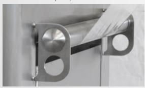
OPEN SLOT DESIGN O-ring gaskets in closed slots create lap joints and dirt traps that are impossible to clean. Open slot design avoids the creation of hidden areas and hygiene is assured with standard cleaning procedures.
