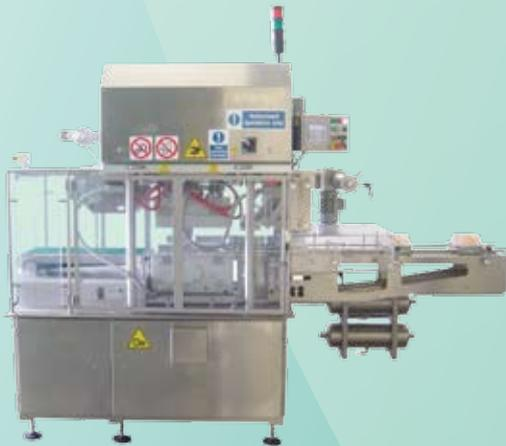
As a guide line, the Rigid Dome kit allows to handle packs up to a maximum height of 110 mm., which can be equally shared between tray and dome. The G. Mondini range includes systems suitable for reaching an output going from 20 trays per minute up to 65 trays per minute designed for this specific application.
